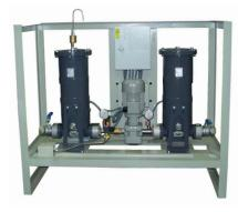
For larger capacity installations and fuel parks the SAFA filtering system guarantees the prevention. For lower flow generators MiniSAFA and MicroSAFA are recommended.
