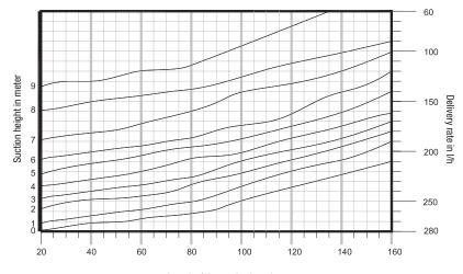
Length of the suction hose in meter Based on factory tests with fuel oil EL at 20°C pipe Ø 22x20
