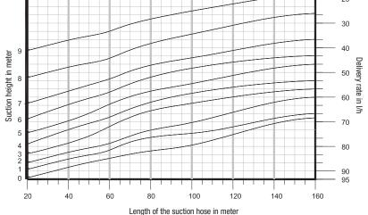
Based on factory tests with fuel oil EL at 20°C pipe Ø 15x13
