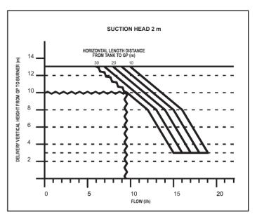
Example: - Suction head between the tank bottom and the desired position for the INPRO MICRO DOMESTIC of 2 m (so please read second diagram above).
