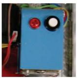
5. Once the light turn off, it will continue operating automatically until the maximun set pressure is reached, which will stop the motor.
